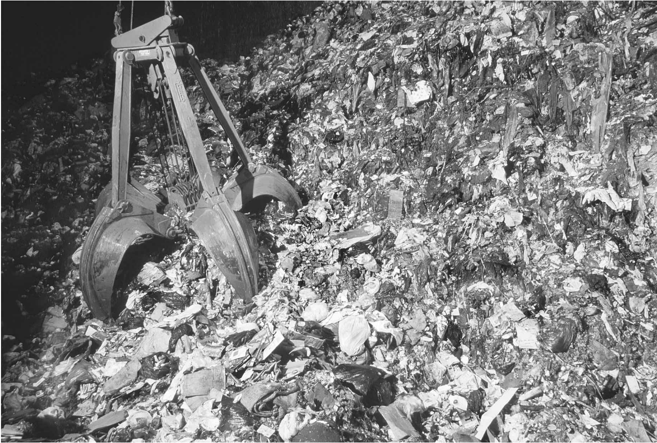
The Bridgeport RESCO power plant mixes garbage to facilitate the drying process, which improves the efficiency of energy generation by incineration. (Corbis Corporation)
