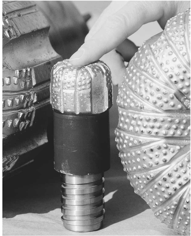
SlimDril drill bits are manufactured from polycrystalline with natural diamonds on the face of the bit for oil and natural gas drilling. (Corbis-Bettmann)
